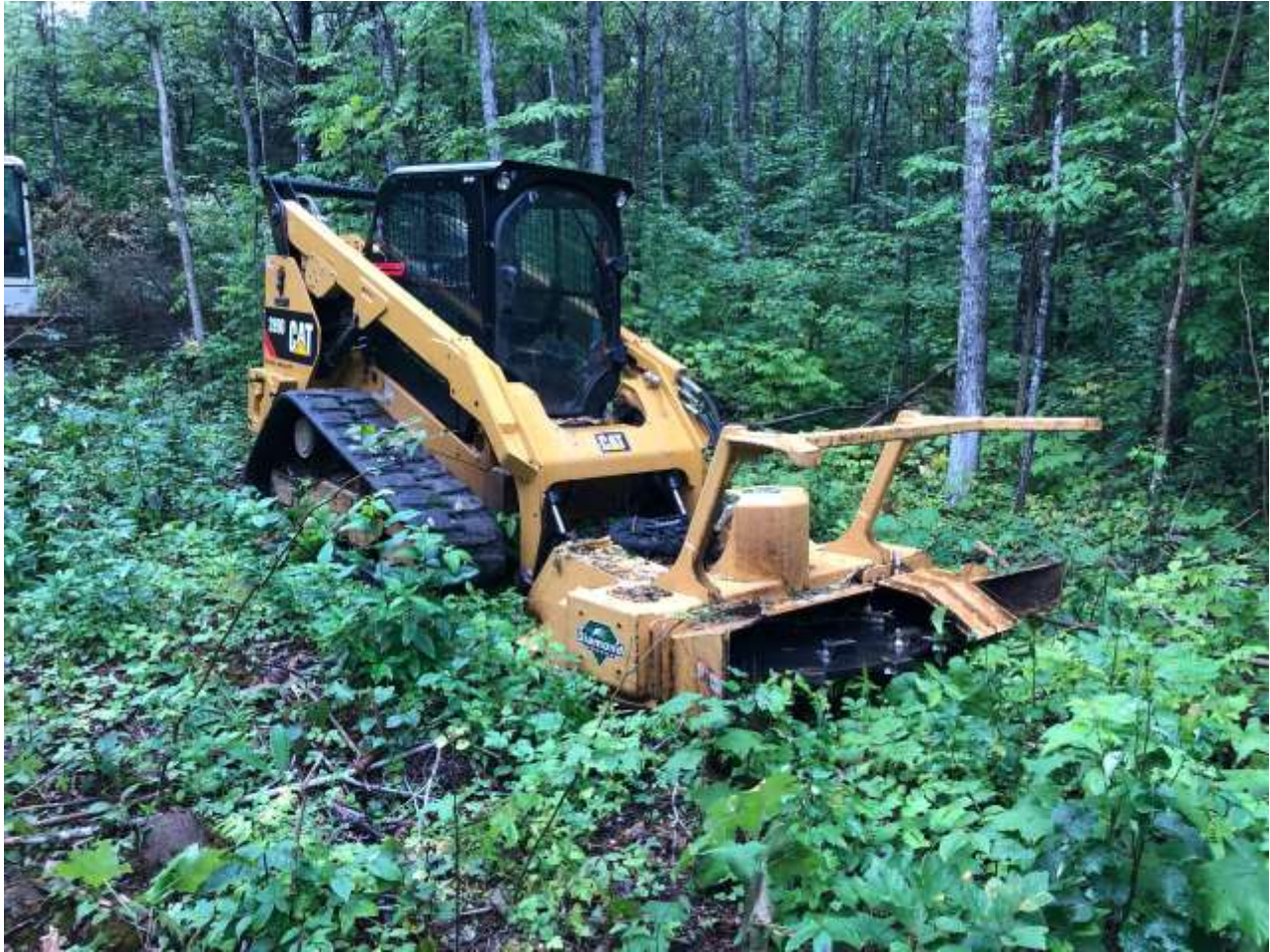
Cat 289 D Skid Steer with the following Attachment Standard Bucket, Grapple Bucket, Articulating Dozer Blade, Power Tiller, Street Sweeper with hopper to capture sweepings, Diamond Mower Brush Shear.
